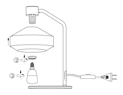
If the external flexible cable or cord of this luminaire is damaged, it shall be exclusively replaced by the manufacturer or his service agent or a similar qualified person in order to avoid a hazard.
