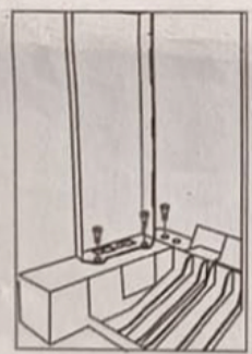
6. STAGE Tighten the mounting screws
