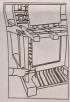
5. STAGE Place pieces 2 on the front and 2 on the back.
