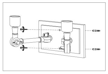
2. Fix the luminaire to your junction box or wall by using suitable wall mounting plugs and screws.
