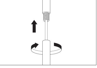
Determine the desired height of the lamp and connect either one, two or three of the pipes supplied. Thread the wire through the pipes.
