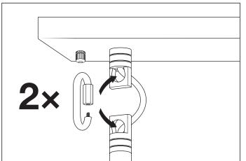
Link the lamp to the canopy using the chain link. Securely close the chain link once the lamp is linked to the canopy.
