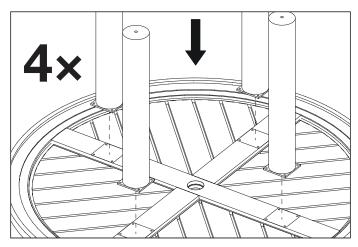
Carefully place the legs on the table top and align the holes of the legs with the holes in the table top.
