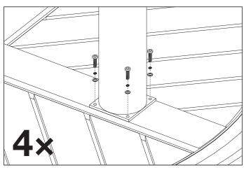
2. Fix the legs onto the table top by securing the screws with an allen key.
