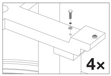
**4.** Fix the foot frame onto the legs by securing the screws with a wrench.
