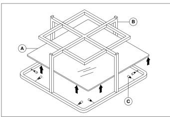
**2.** One person should hold the glass in an elevated position while the other person places the glass supports.
