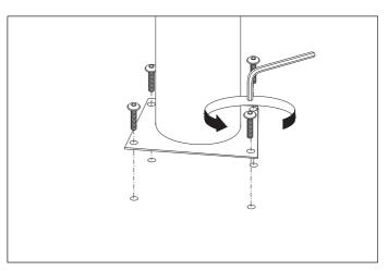
2. Place the legs in the correct position, aligning the holes of the legs with the holes of the top. Fix them with the bolts by using the provided allen key.
