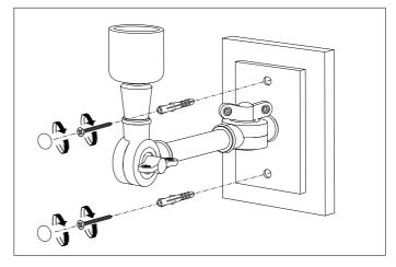
${\bf 2.}$  Fix the luminaire to your junction box or wall by using suitable wall mounting plugs and screws.
