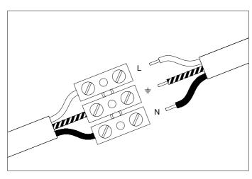
1. Connect the 3 wires according to their colours. Brown is the live wire (L), blue is the neutral wire (N), green/yellow is the earth wire  $(\frac{L}{m})$ .
