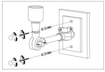
$\textbf{2.} \ \mathsf{Fix} \ \mathsf{the \ luminaire \ to \ your \ junction \ box \ or \ wall \ by \ \mathsf{using \ suitable \ wall \ mounting \ plugs \ and \ screws.}$
