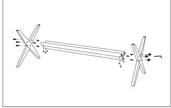
1. Assemble the base as shown in the drawing. See picture 2 for a detailed view.
