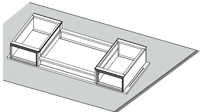
**3** Assemble the legs from the inside with the screws.
