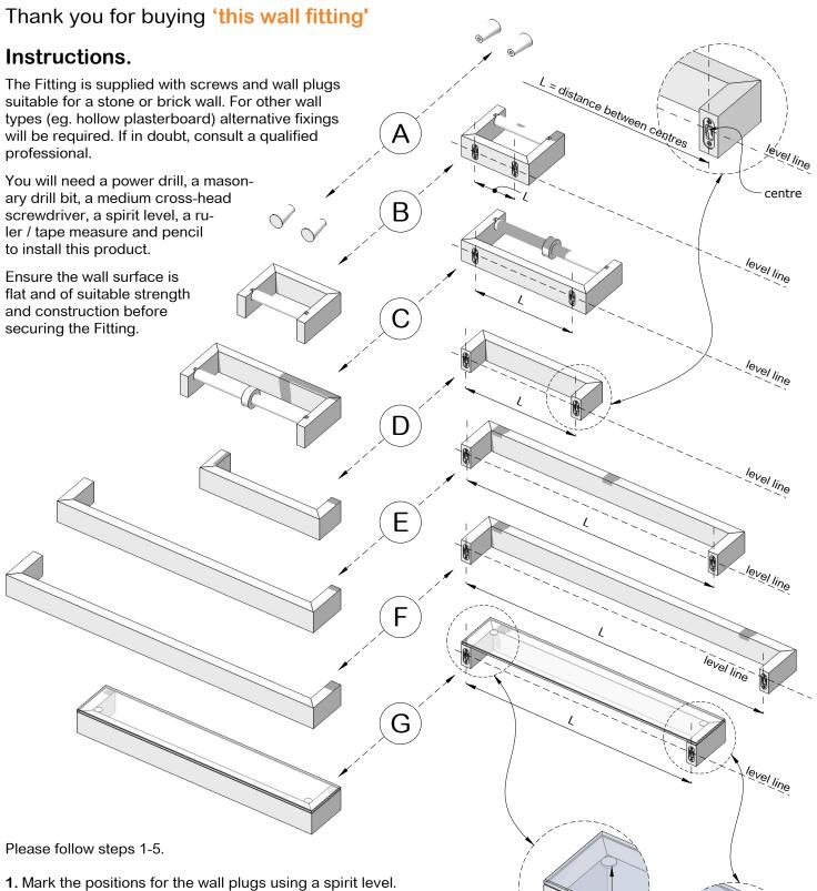
Use the table below to mark out the distance between fixing points (check measurements match actual fitting dimensions)
