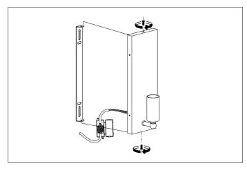
${\bf 3.}$  Place the wall plate over the crossbar and fix it securely with the screws supplied.
