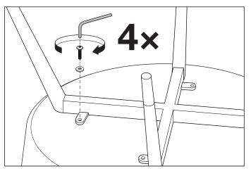
2. Fix the frame to the base using the allan screws combined with the metal rings. Secure the screws tightly before using the chair.
