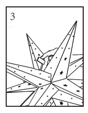
3. Fix the LED set in the star by using the plastic clip.
