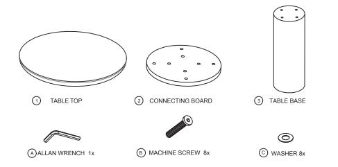
"First loosley assemble all the screws into all the parts. After loosley fitting all screws, proceed to tighten them firmly to secure the whole construction."
