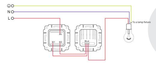
**2.3 Connection of two dimmers to a pass-through circuit** This diagram option is used when not only switching but also light intensity control from two locations is required. Note that this requires two identical dimmers. In such a circuit, pass-through dimmers should be used.
